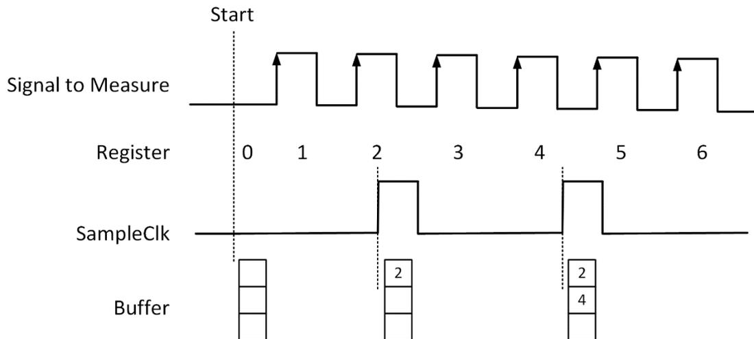
Figure 56 Buffered Edge Counting with Internal Sample Clock
