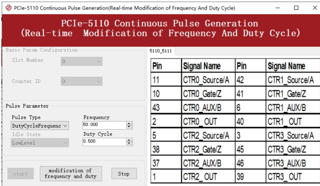
Figure 101 Continuous Pulse Generation
