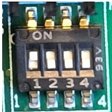
Figure 104 DIP switch in PCIe-5111
