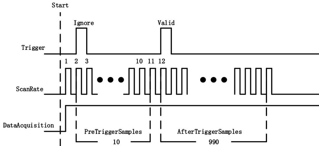
Figure 28 Reference Trigger
