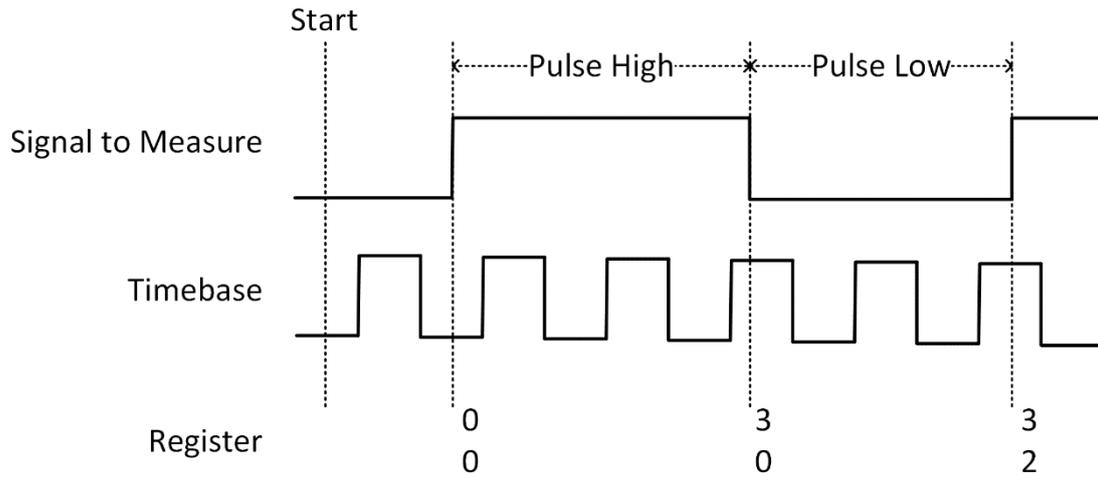
Figure 63 Pulse Measurement in Single Mode
