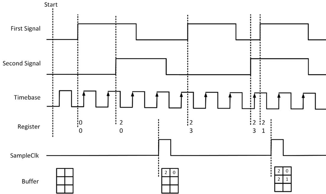
Figure 77 Two-Edge Separation with Internal Sample Clock
