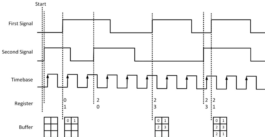
Figure 78 Two-Edge Separation with Implicit Sample Clock
