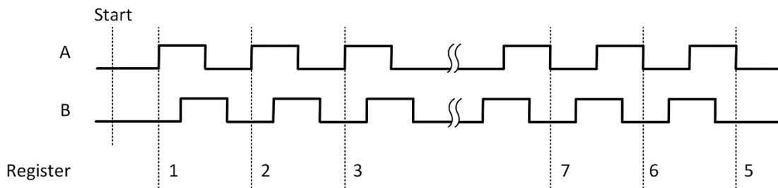
Figure 81 Quadrature Encoder x1 Mode
