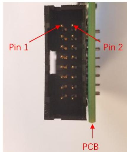
Figure 103 SSI Connector in PCIe-5111
