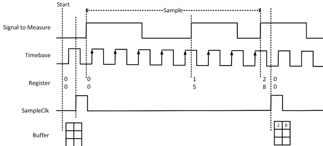
Figure 70 Frequency Measurement with Internal Sample Clock
