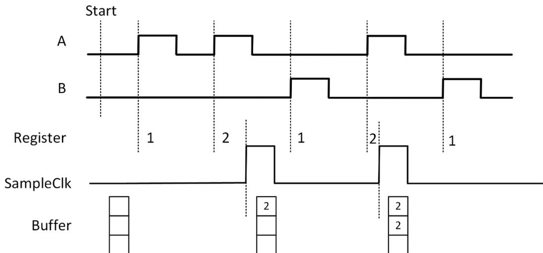
Figure 89 Two-Pulse Encoder with Internal Sample Clock
