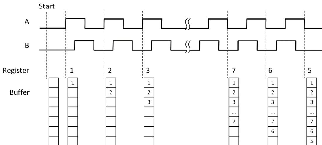
Figure 85 Quadrature Encoder x1 with Implicit Sample Clock
