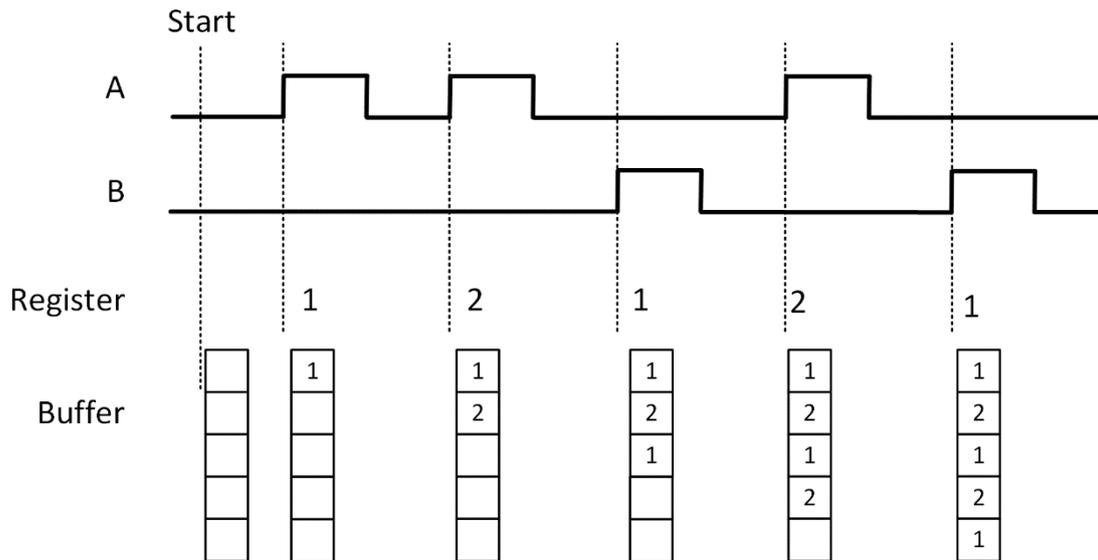
Figure 90 Two-Pulse Encoder with Implicit Sample Clock
