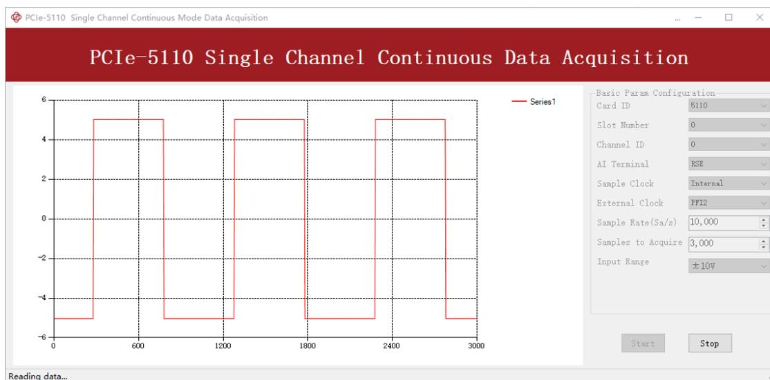
Figure 43 AI Acquisition AO Square Signal
