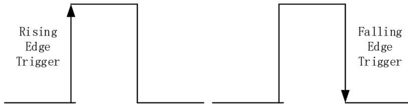
Figure 24 External Digital Trigger
