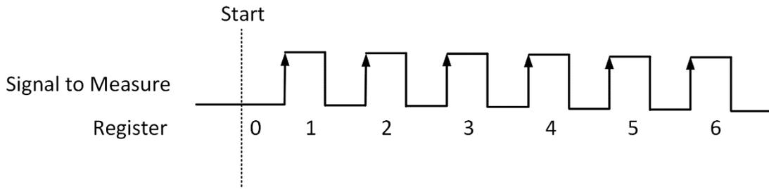
Figure 55 Simple Edge Counting in Single Mode
