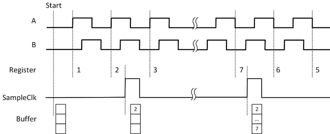
Figure 84 Quadrature Encoder x1 with Sample Clock
