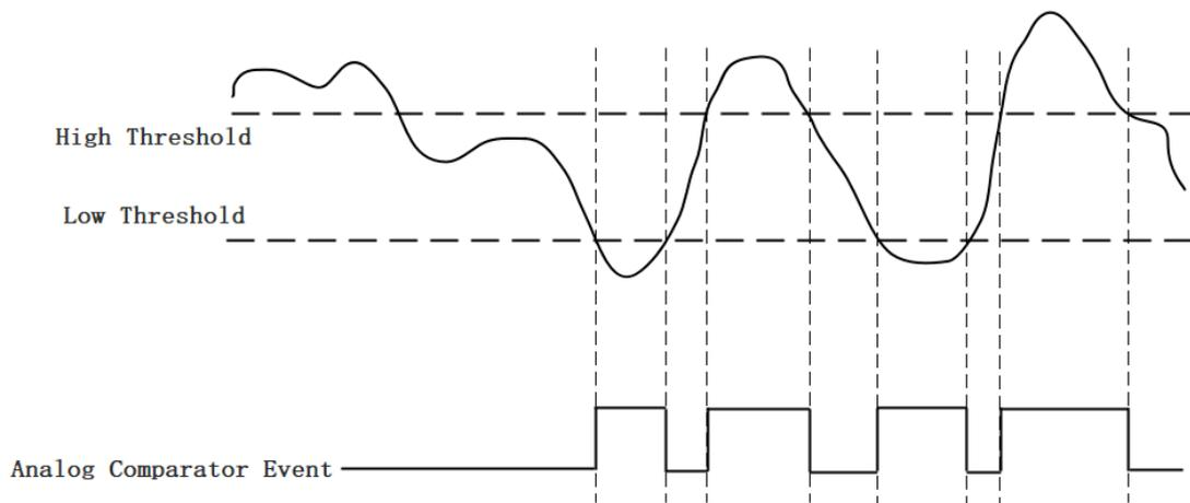
Figure 20 Leaving Window Trigger
