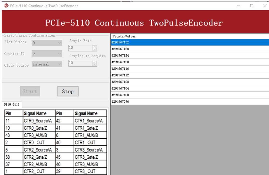
Figure 93 Two-PulseEncoder For Continuous Mode
